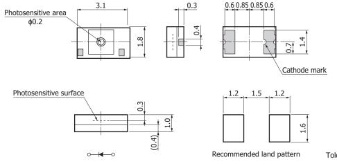
Position accuracy of photosensitive area: X,  $Y \le \pm 0.2$
