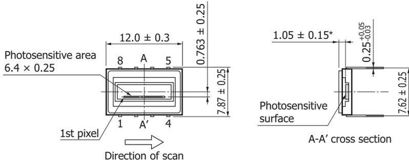
\* Distance from upper surface of window to photosensitive surface
