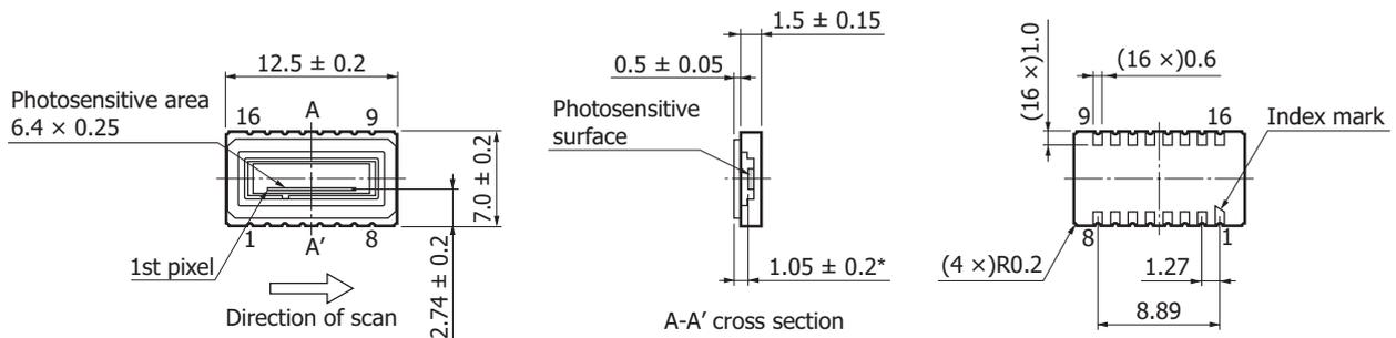
\* Distance from upper surface of window to photosensitive surface
