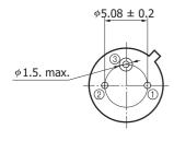
Distance from photosensitive area center to cap center  $-0.3 \le X \le +0.3$   $-0.3 \le Y \le +0.3$
